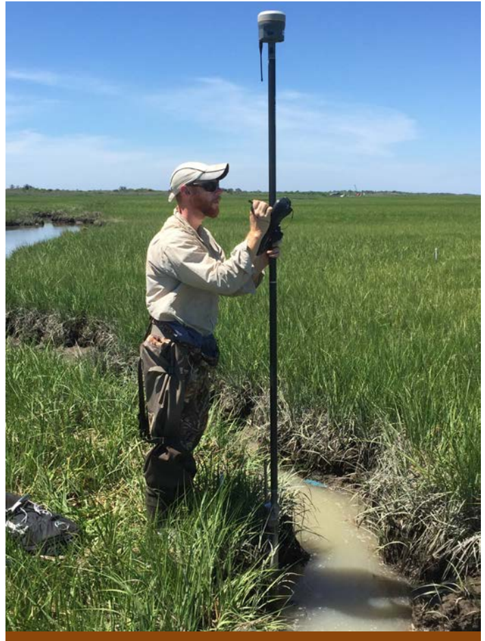
Andrew Neil, a cooperater at the University of Rhode Island, collects elevation along a ditch at Fire Island National Seashore. Points were established using a 20-m grid which covers the range of elevation and vegetation types in the salt marsh. NPS
